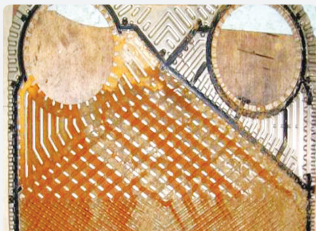
BEFORE & AFTER PLATE HEAT EXCHANGER CHEMICAL CLEANING
